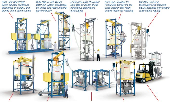
Bulk Bag Unloader for Pneumatic Conveyors has surge hopper with non-flowthrough pick-up adapter
